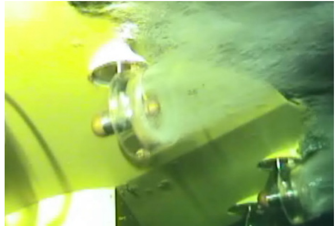
An example of thruster ventilation test in a sea way
